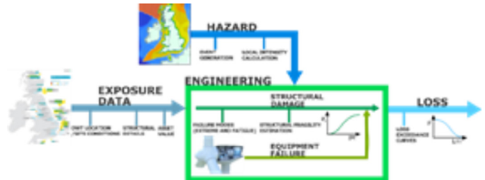
Figure 1: Proposed probabilistic risk modelling framework for offshore wind turbines
