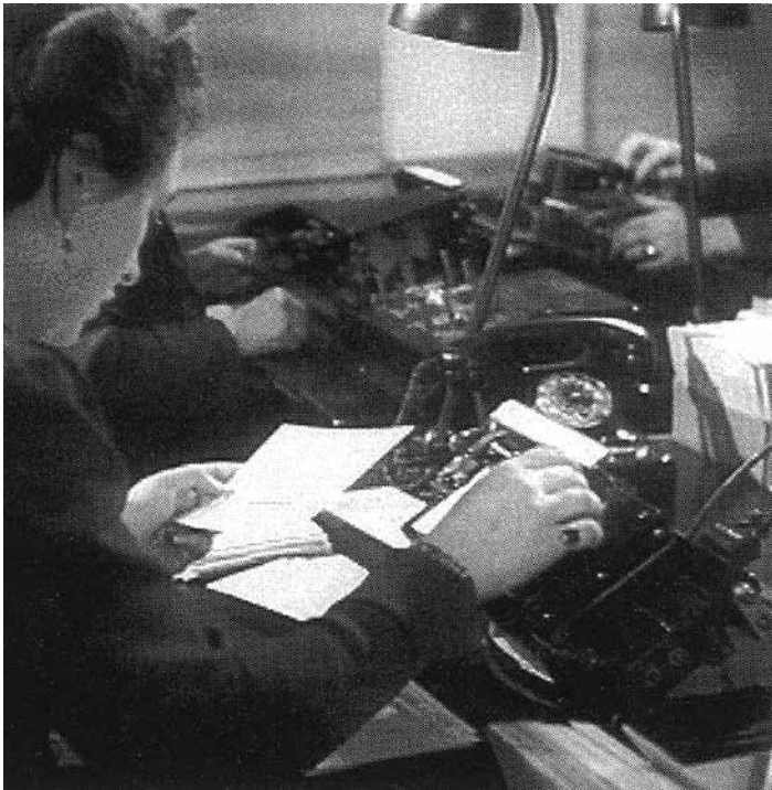
The hand punch card device was used to transfer statistical data to the punch card (film print).
