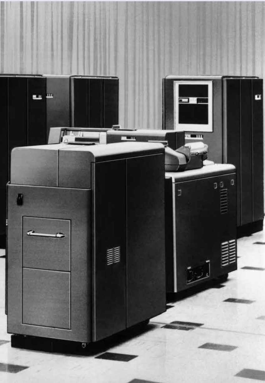
The IBM 650 magnetic drum computer from 1953 with the corresponding punch card devices.
