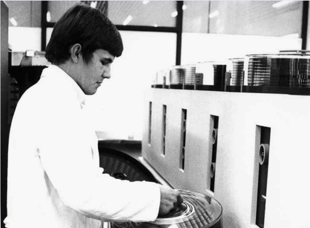
In a disk storage unit, up to eight magnetic disk storage units could be used simultaneously. In the picture: Johann Knöferl.
