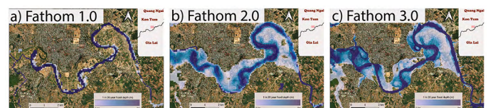
Figure 1: Flood hazard map of Kon Tum, Vietnam, for the one in 20-year flood event. Three versions of a Global Flood Model (GFM) courtesy of Fathom, each with a different underlying elevation dataset, were compared. Panel a) uses the SRTM elevation dataset, Panel b) uses MERIT DEM, and Panel c) uses FABDEM. Note the improved delineation of floodplain features in panel c).
